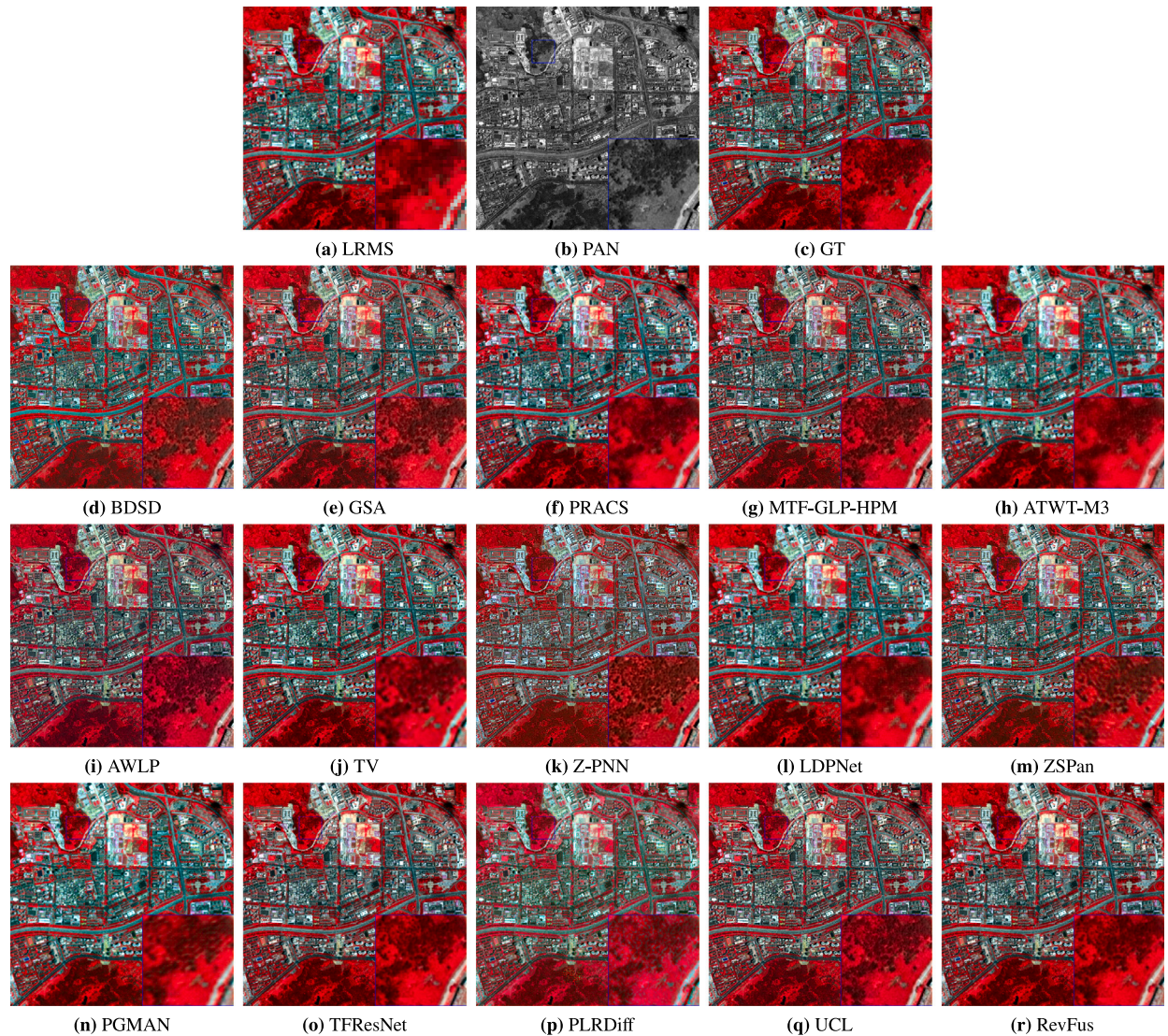
Fig. 5. Visual comparison of pan-sharpening methods on the QuickBird dataset in the reduced-resolution testing scenario. The results are displayed in false-color, where bands 4, 3, and 2 correspond to the RGB channels.
