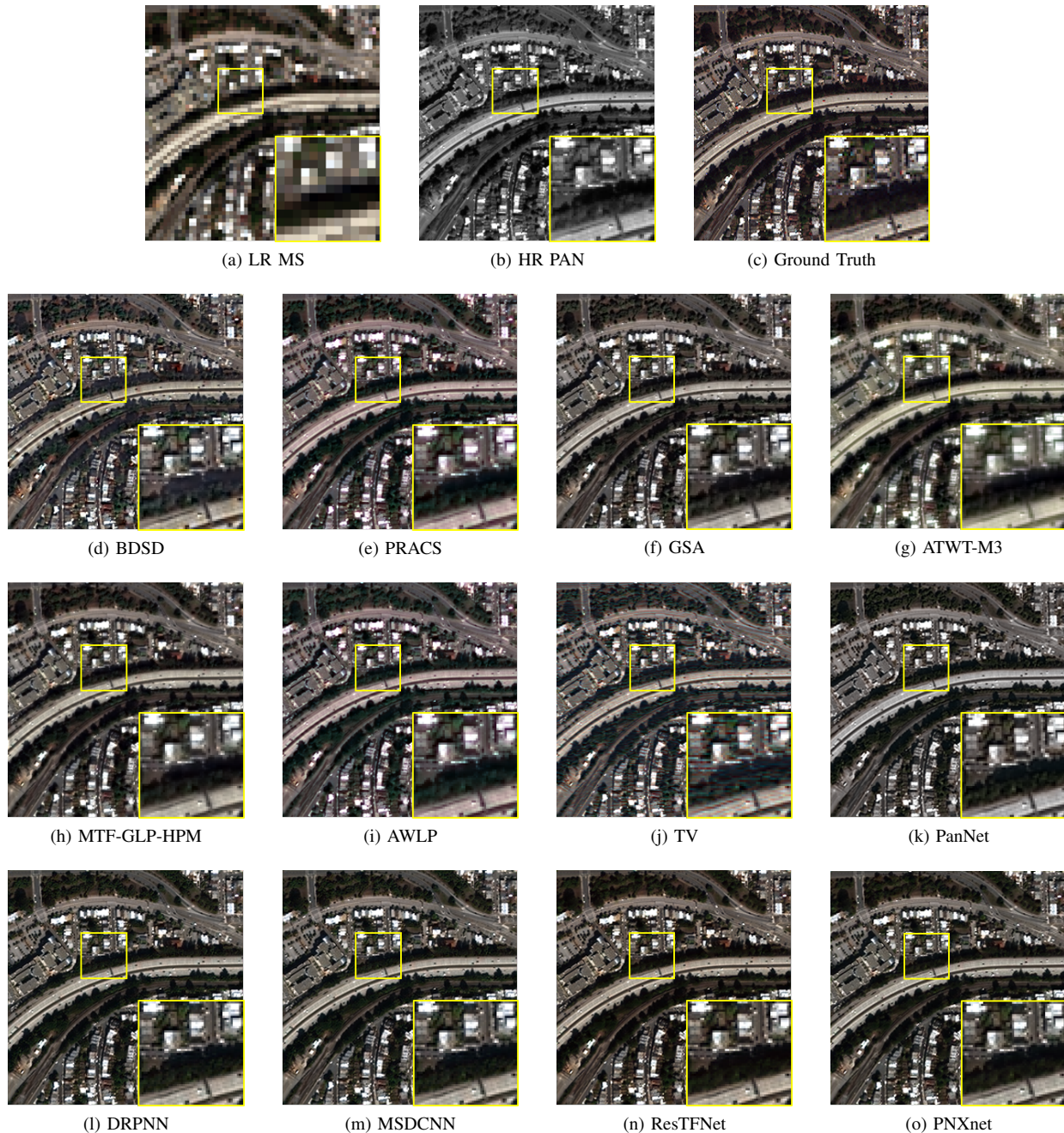
Fig. 7: Pan-sharpening results on WorldView-2 images. Enlarged views are shown in yellow box. The first row shows input data and ground truth. Row 2 to 4 present the results of comparison methods and the proposed PNXnet.
