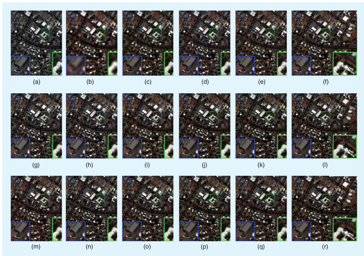
FIGURE 15. Visual comparisons in natural colors of the evaluated approaches on the reduced-resolution WV4 Alice Springs data set (see Figure 11). The (a) PAN, (b) EXP, (c) BT-H, (d) BDSD-PC, (e) C-GSA, (f) SR-D, (g) MTF-GLP-HPM-R, (h) MTF-GLP-FS, (i) TV, (j) PanNet, (k) DRPNN, (l) MSDCNN, (m) BDPN, (n) DiCNN, (o) PNN, (p) A-PNN-FT, (q) FusionNet, and (r) GT.
